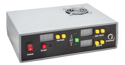
POWER switch – turns the driver on / off
