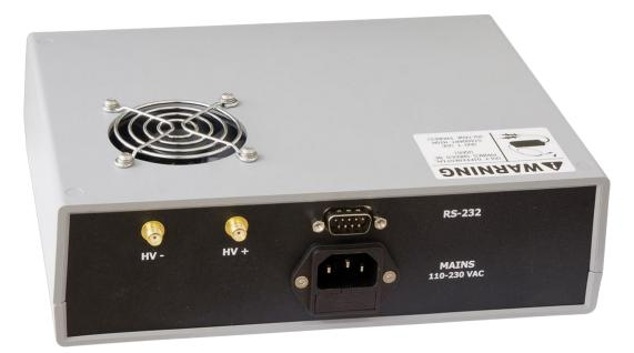
In this version, 1000V voltage set point means that +500V (relatively to the ground) will be delivered to HV+ SMA connector and -500V (relatively to the ground) will be delivered to HV- SMA connector. One connector or both can be used at the same time. 23pF maximum load capacitance can be connected to HV+ and/or HV- connectors.
