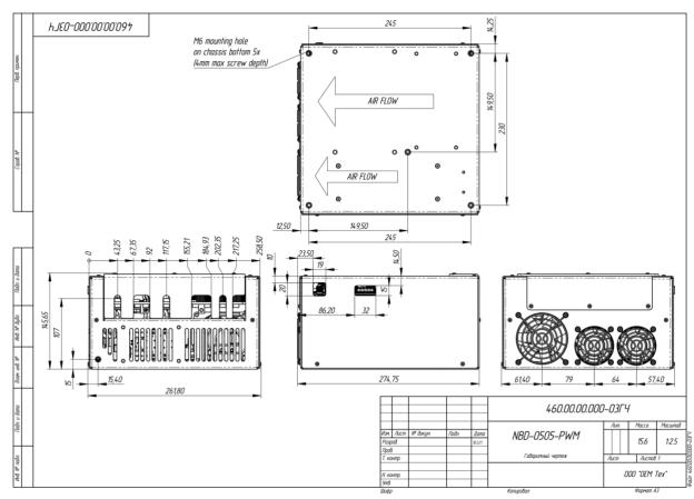
Non-optimal air flow direction in this option might result in reduced maximum average power.
