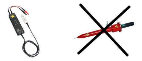
In terms of performance, please keep in mind, that differential probes have significant capacitance, which should be counted as a part of the load capacitance.
