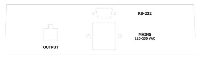
MAINS connector (cable is supplied with the module) – connects module to the mains (110/230 VAC, 50/60 Hz). This connector contains 5A fuse.
