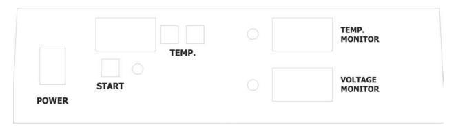
POWER switch – turns thermo controller on and off TEMP. indicators – depict the temperature set points TEMP. buttons – change the temperature set points
